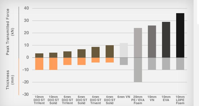
Impact Energy: 10J The lower the Peak Transmitted Force, the higher the impact protection
